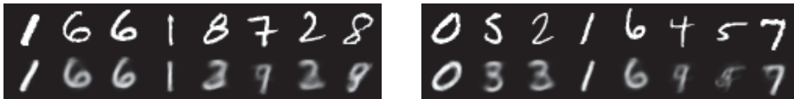
Figure 5.10: Images x on the top row and its reconstruction \mu_x(q_\varphi(x)) on the bottom row produce from a simple VAE with latent space of dimension d = 2 and \sigma = 1
