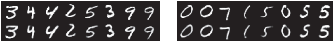
Figure 5.14: Images x on the top row and its reconstruction \mu_x(q_\varphi(x)) on the bottom row produced from a simple VAE with latent space of dimension d = 20 and \sigma = 0.0001
