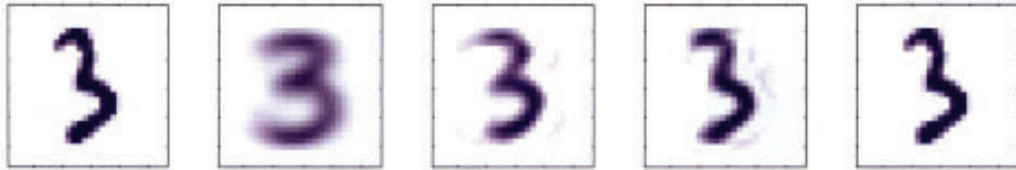
Figure 5.6: Examples of reconstruction produced by PCA included in Bishop’s book [15]. The image to the left is a real image and other images are reconstruction with latent space of size d = 1 , d = 10 , d = 50 and d = 250 respectively.
