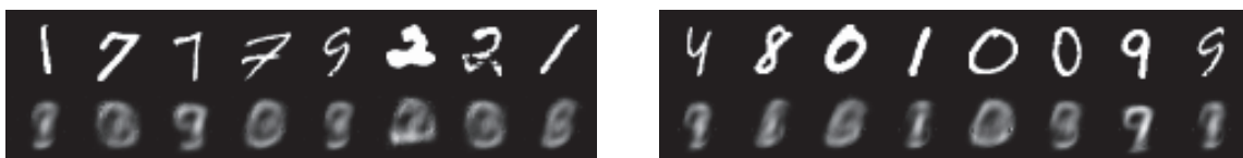
Figure 5.4: Images x on the top row and its reconstruction \mu_x(q_\phi(x)) on the bottom row produce from a simple VAE with latent space of dimension d = 2
