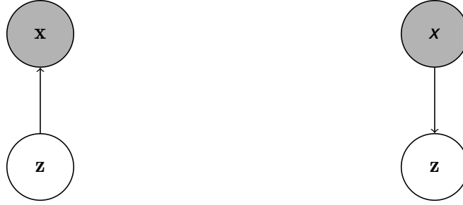
(a) Generative network. It assumes p(\mathbf{x}, \mathbf{z}) = p(\mathbf{z})p(\mathbf{x}|\mathbf{z}) . (b) Inference network. Given observations \mathbf{x} we can infer the latent variable using q(\mathbf{z}|\mathbf{x}) .
